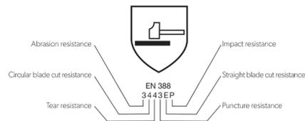
For gloves that do not meet the minimum requirements of level 1 for each element, a 0 is typically displayed. The EN388 rating for a nitrile examination glove would most likely be 0000X.
